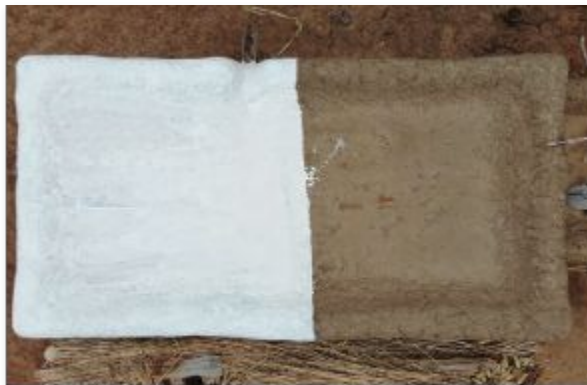
Coated (left) Vs. uncoated (right) roof
